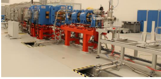
Figure 2. The full transport section of the ELIMED ion beam
