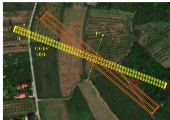
Figure 1. Intersection of the 110 kV and 400 kV overhead lines
